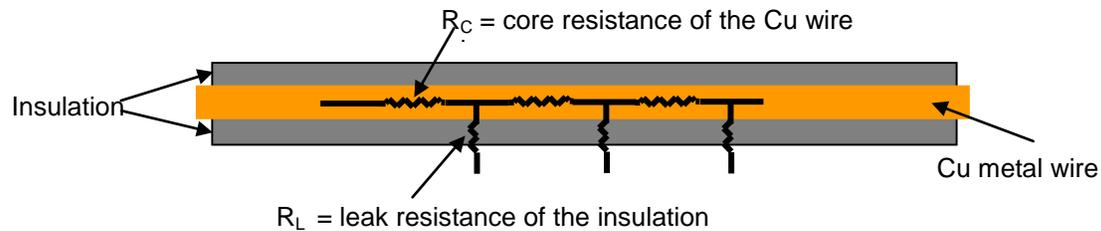
Figure 5: Cross section of an insulated metal wire.
