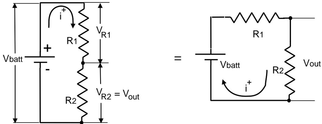
Figure 2: Two equivalent representations of a voltage divider.
