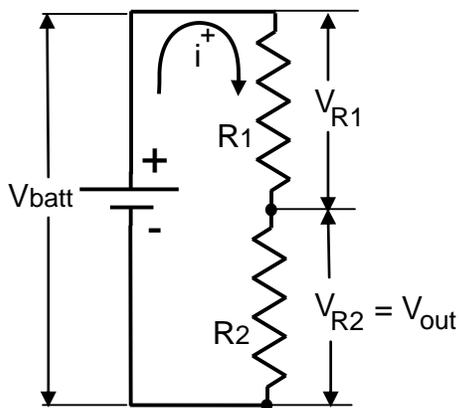
Figure 1. A simple voltage divider. Positive current ( $i$ ) flows from the positive pole of the battery through two resistors in series to the negative pole of the battery.
