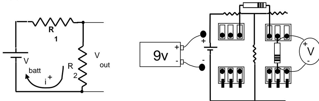
Figure 7. Voltage divider circuit and project board wiring diagram.
