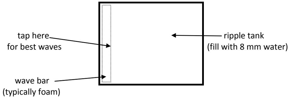
Pour water in the ripple tank so that it is about 8 mm deep. Turn on the light.
