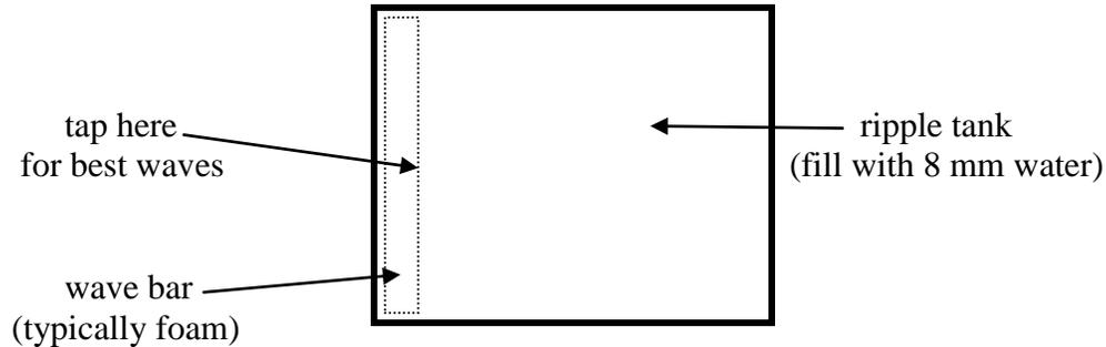
Pour water in the ripple tank so that it is about 8 mm deep. Turn on the light.
