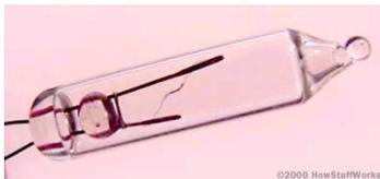
15. A typical strand of 50 mini-lights has lamps that are rated at 2.5V each. If a household circuit is 120V, why are the mini-lights wired in *series*? HINT: 48 would be a perfect number of mini-lights to wire in *series* for maximum effect. (Refer to the *Electricity* page on your Physics reference table.)
